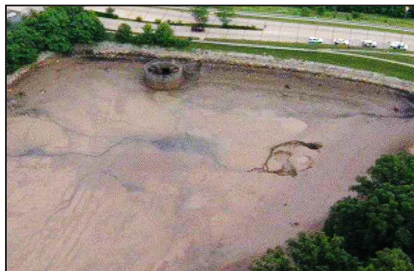
Figure 6B Post-collapse aerial view of Lake Chesterfield showing sinks that formed at the cave beneath the lake.
